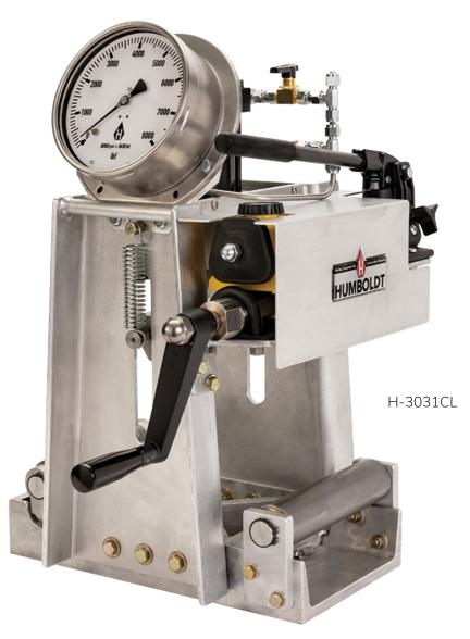
The Humboldt H-3031CL Portable, Continuous-Load, Concrete Beam Breaker is a great quality control tool for contractors, DOTs and consultants for quickly and accurately determining flexural strengths of concrete using 4" x 4" x 14" test beams.
